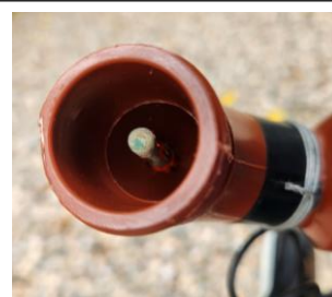
View of the thermometer bulb inside the elbow.
