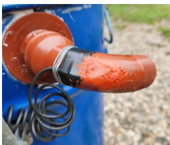
Outlet elbow with the thermometer bulb inside.
