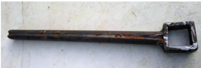
Nozzle-cleaning rod with a groove for the water drops
