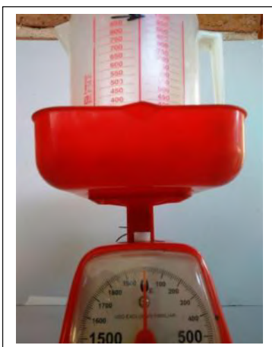
Adjust the scale to zero with the empty jar on it.
