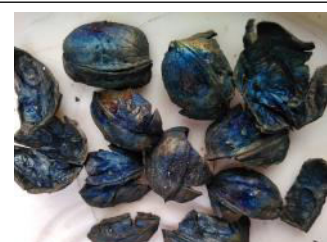
Ph.8: The result : Blue Charcoal, crystal sounding, no tar.
