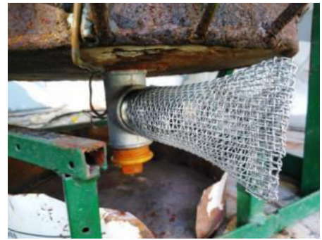
Flame arrestor at the port. Tray placed under the nozzle.
