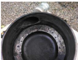
Original air inlet holes plugged and the new tangential inlet pipe welded.
